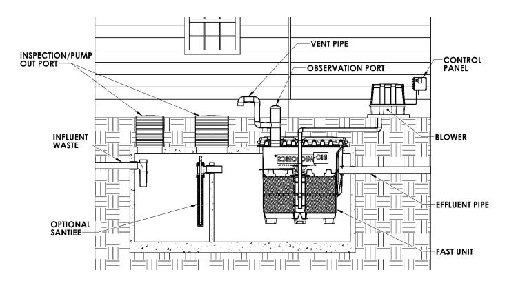
**Shown:** A MicroFAST unit installed with the lid option. Consult your Installation or Service Manual for representations of other units covered by this Owner's Manual.
